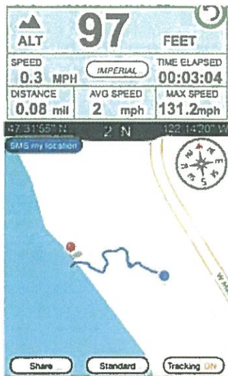
Figure 2.0 – GPS Altimeter reading at the southeast property corner – 97' elevation
